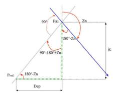
The factor C: on the figure above is a detail of the plot we see that Dep =  $\Delta l \times \cot Z$ n As  $\Delta g = Dep \times \sec l$  then  $\Delta g = \Delta l \times \cot Z$ n sec  $l = C \times \Delta l$ . As C=See definition of C in formularies.
