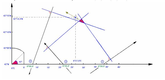
Transfer the position triangle over 2,2 M at 301° in order to correct the error due to nutation of the earth's axis.
